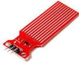
**Figure.1.7: Image of Water Level Sensor**
